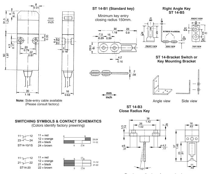
For close radius keys for mounting key close to (within 50 mm) door hinge, order ST 14-B3.
