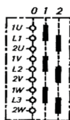
▲ ▲ 2 Speed, 2 Winding (OFF-LOW-HIGH)
