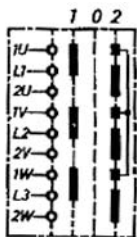
▲ 2 Speed, 1 Winding (LOW-OFF-HIGH)
